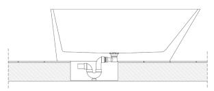
12. Fill the bathtub with water to check that all water flows freely to the waste outlet.
