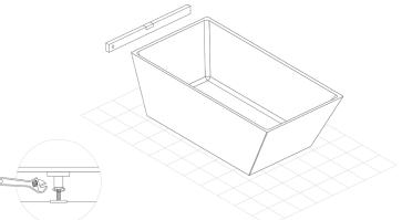
**\*\*IMPORTANT**\*\* - Water will only drain properly to the waste outlet if the bathtub is level.
